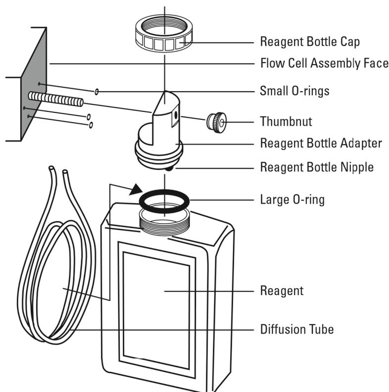
Figure 10: Reagent Bottle Assembly
