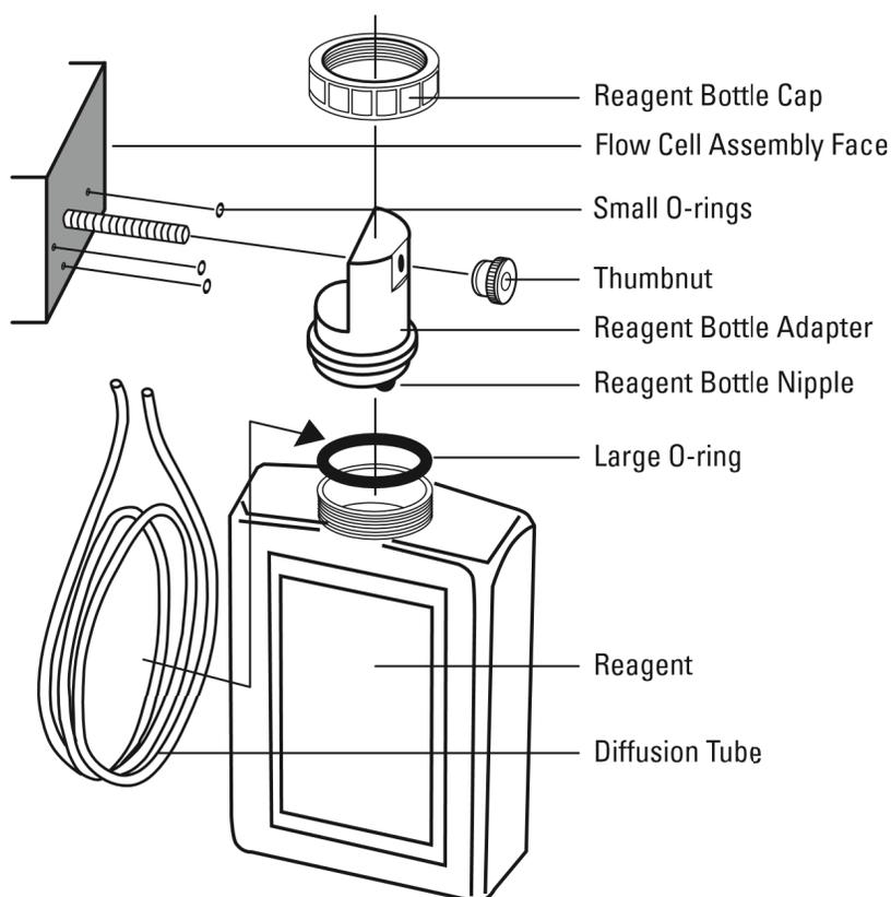
Figure 21: Reagent Bottle Assembly
