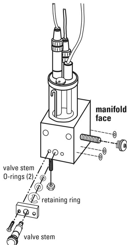
Figure 22: Flow Cell Assembly
