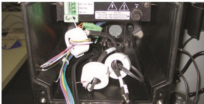
Figure 11: Ferrite Installation
