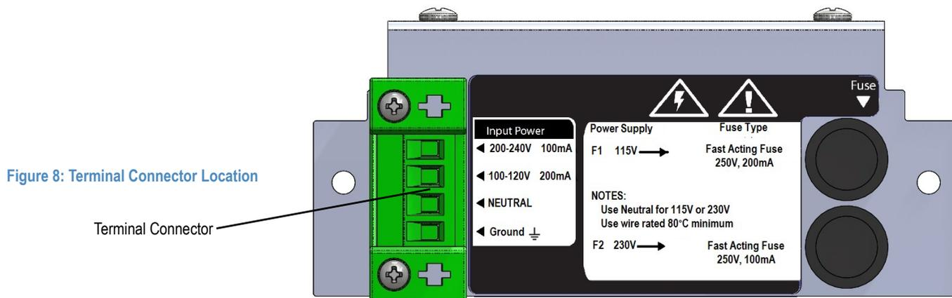
5. Wire the power cable to the green screw terminal connector from the options kit. Select correct terminal for hot conductor depending on line voltage, insert ground wire into the correct terminal and connect the other cable to the neutral terminal. Refer to Figure 8 for terminal connector location.
